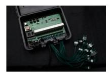
A 16-channel, 110-volt AC dimmable controller that allows control of LED or Incandescent Light Strings at up to 2 amps per channel. Control lights via our NEC, a standard *DMX*-512 lighting console, or computer using *DMX* software like *Xlights* or other *DMX* compatible software. Used with *Xlights*, the Express allows the user to combine RGB and non-RGB light elements in a cohesive show.
