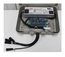
Rainmin's Network Distribution Boxes boxes are the bridges from your *ArtNet*, *sACN* or NEC controllers to our intelligent light strings. This 4-port version comes with on-board power and a weatherproof box. Connect multiples with unique IP addresses via third-party network switch. Input up to 16 *ArtNet* universes across 16 ports.
