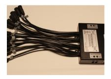
Ethernet controller for RGB light strings. Works with our Network Effects Controller or with most *ArtNet* and *DDP* compatible software or hardware controllers. Distributes power and data to light strings. 16 outputs with 10 inch pigtails. Can also be used with Smart-Ts.
